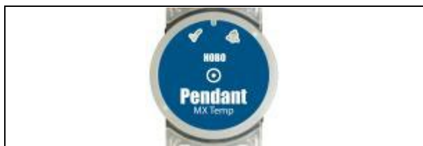
Special Sensors were placed under the ice to record water temperatures at the bottom of the river channel
