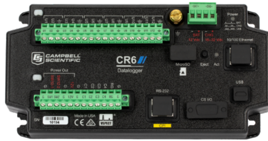
Fig. 2. Panel a) is open-source electronics prototyping platform (Arduino; By SparkFun Electronics from Boulder, USA - Arduino Uno - R3, CC BY 2.0, https://commons.wikimedia.org/w/index.php?curid=26785892 ) which relies on open-source programming and peer-to-peer sharing. Panel b) is a proprietary datalogger platform (model Cr6 Campbell Scientific Inc.; https://www.campbellsci.com/cr6 ) which is supported by the company's manufacturers. In general, panel b) is the best choice for project teams that has limited experience with dataloggers.
