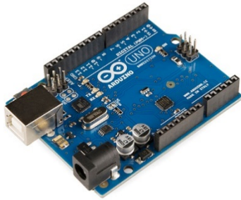
Fig. 2. Panel a) is open-source electronics prototyping platform (Arduino; By SparkFun Electronics from Boulder, USA - Arduino Uno - R3, CC BY 2.0, https://commons.wikimedia.org/w/index.php?curid=26785892 ) which relies on open-source programming and peer-to-peer sharing. Panel b) is a proprietary datalogger platform (model Cr6 Campbell Scientific Inc.; https://www.campbellsci.com/cr6 ) which is supported by the company's manufacturers. In general, panel b) is the best choice for project teams that has limited experience with dataloggers.
