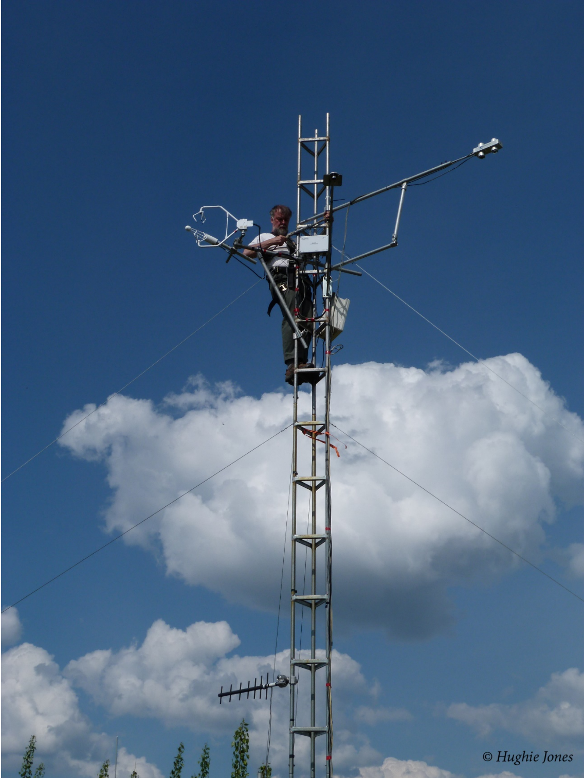
Fig. 13. Example of climate station supported by a triangular tower.
