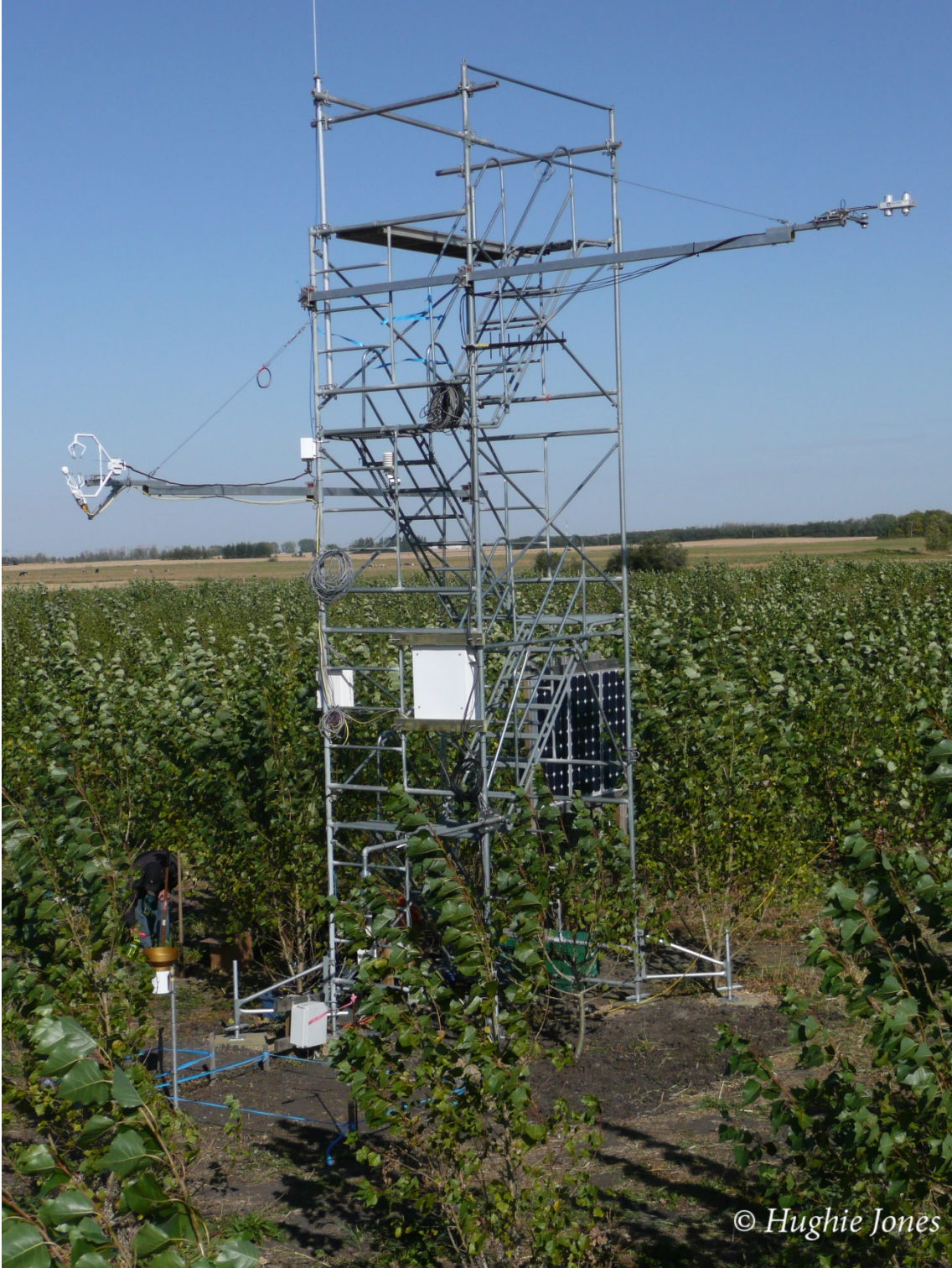
Fig. 12. Example of climate station supported by a scaffold tower.
