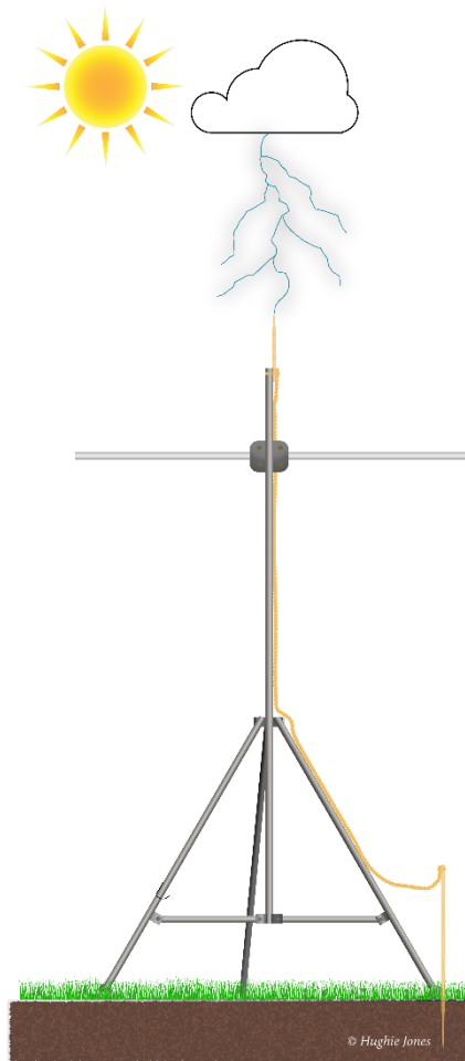
Fig. 9. Illustration of climate station infrastructure and lightning protection equipment necessary to ground the climate station
