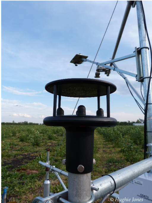
Fig. 6. Panels a) is a picture of a sonic anemometer used to measure wind speed and direction. Panel b) is an illustration of a sonic anemometer, as seen in Fig. 1 .
