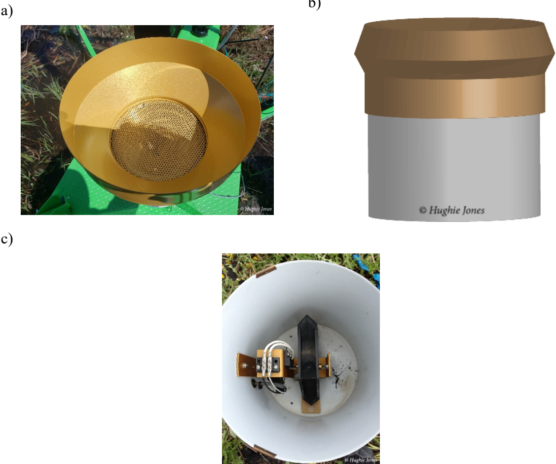
Fig. 3. Panel a) is a picture of a tipping bucket rain-gauge, with a debris screen. Panel b) is an illustration of a tipping bucket rain-gauge, as seen in Fig. 1. Panel c) is an overhead view of a tipping bucket rain-gauge with the rainfall catcher and debris screen removed, which shows the tipping bucket and associated electronics.
