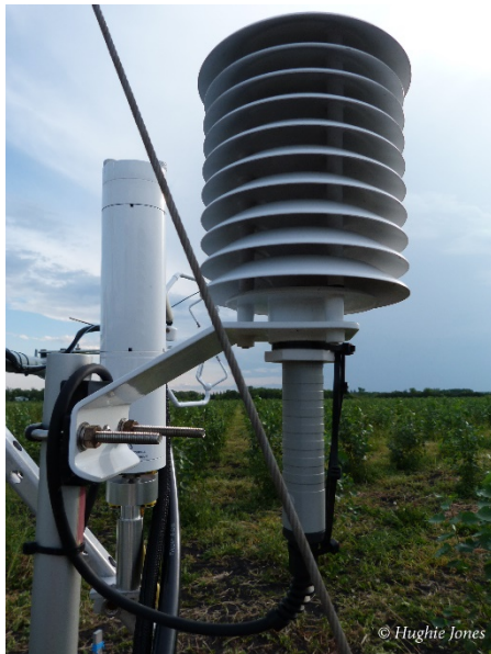
Fig. 4. Panel a) is a picture of a radiation shield with an air temperature and relative humidity sensor extending from the bottom of the shield. Panel b) is an illustration of a radiation shield and the air temperature and humidity sensor side by side, as they would appear separate from one another. The illustration in panel b) is used in Fig. 1 .
