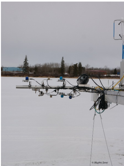
Fig. 8. Panels a) is a picture of a quantum sensors used to measure as photosynthetic flux density (PPFD). The upward facing sensors measure incoming PPFD and the downward facing sensors measure PPFD. Panel b) is an illustration of quantum sensors, as seen in Fig. 1 .
