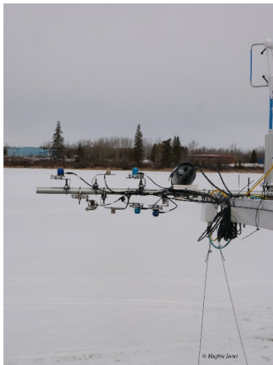
Fig. 7. Panels a) is a picture of pyranometers and pyrgeometers used to measure shortwave and longwave radiation, respectively. The upward facing sensors measure incoming radiation and the downward facing sensors measure outgoing radiation. Panel b) is an illustration of a pyranometers and pyrgeometers, as seen in Fig. 1.
